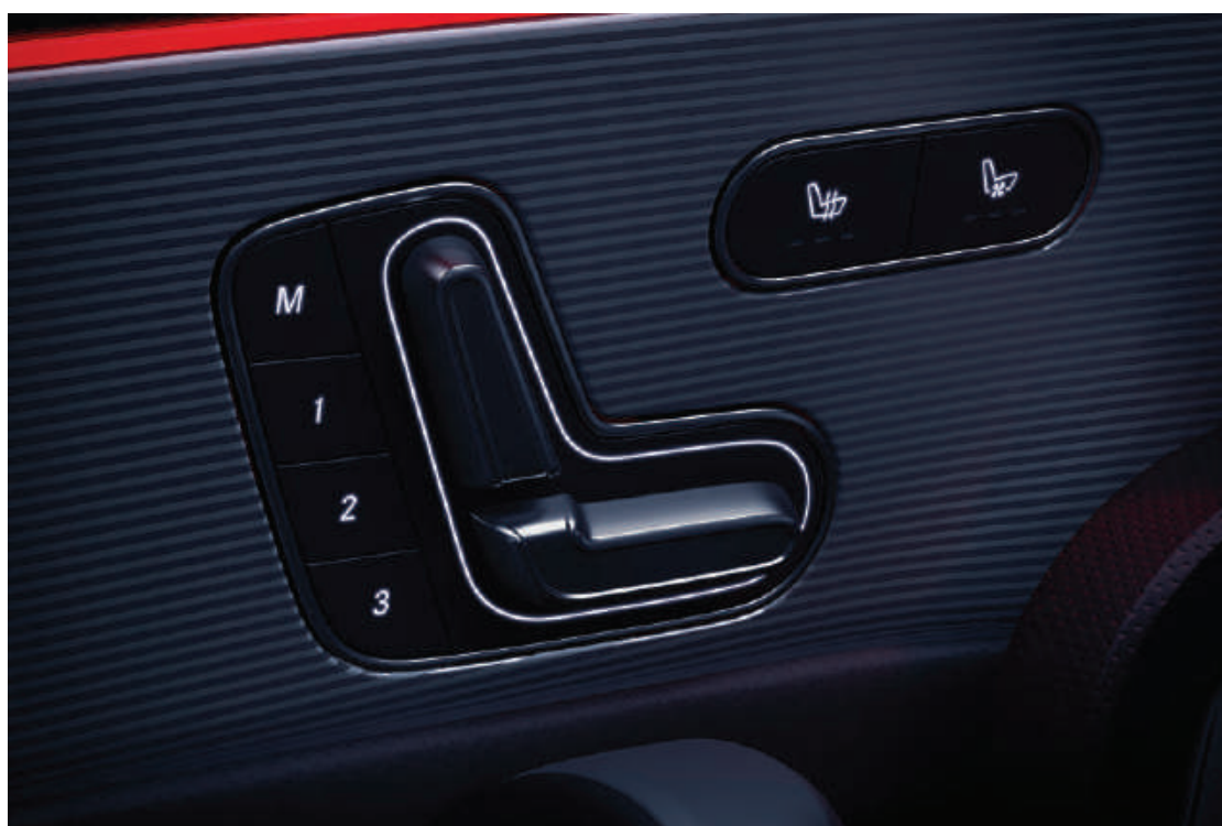
Electrically adjustable front seats with memory function
