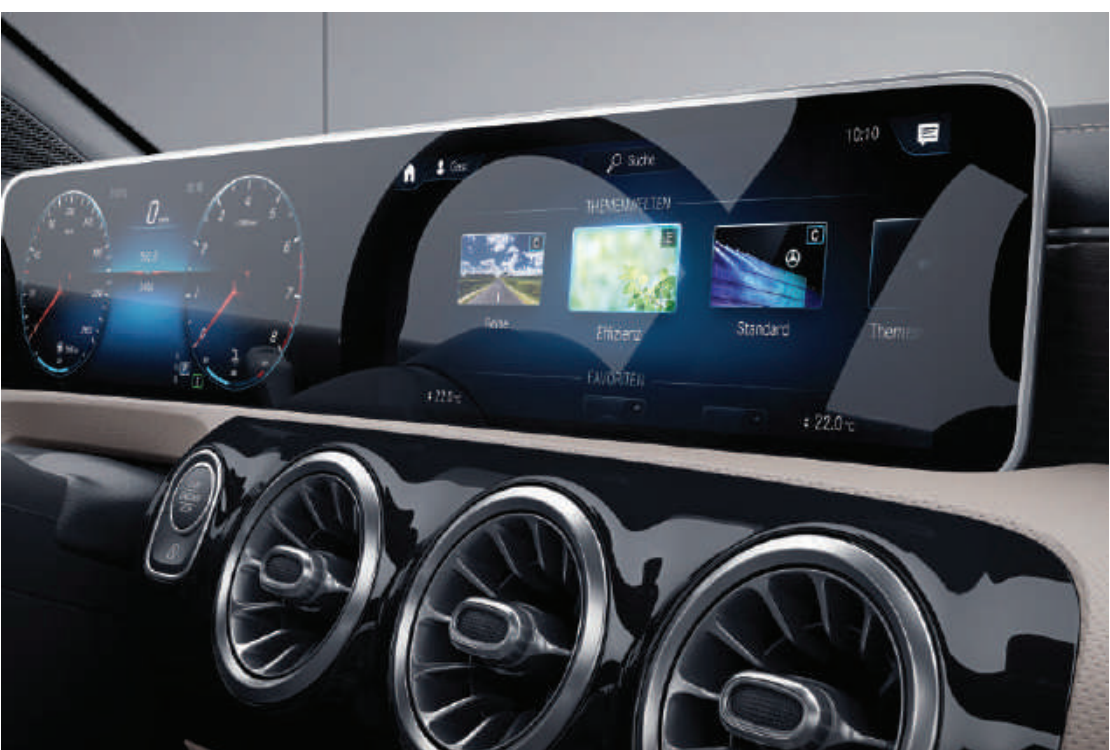
Widescreen cockpit (2 x 10.25-inch display)
